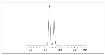
**Figure 6.**Separation of 2,4,5-trichlorophenol and 2,4,6-trichlorophenol isomers with mass 196.
