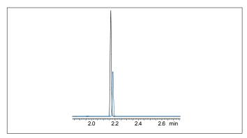
ZB-SemiVolatiles also provides separation for key pairs of analytes that may have similar ions in common. The example of aniline and bis(2-chloroethyl)ether whose main ions are mass 93 are shown in **Figure 5**. Another critical separation is between the 2,4,5-trichlorophenol and 2,4,6-trichlorophenol isomers which share mass 196 as shown in **Figure 6**. Both sets of compounds here exhibit baseline separation on the ZB-SemiVolatiles column.
