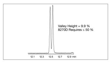
The power to separate PAHs also extends to the last pair of PAHs, indeno[1,2,3-cd]pyrene and dibenz[a,h]anthracene. Though the main ions of these compounds are different, dibenz[a,h]anthracene contains a strong mass 276 which is the main ion for indeno[1,2,3-cd]pyrene. It is therefore desirable to chromatographically separate these compounds to meet the method requirements for compounds with similar masses.
